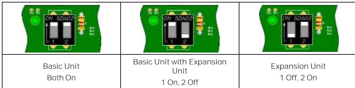
Figure 12. Backplane DIP Switch Settings
