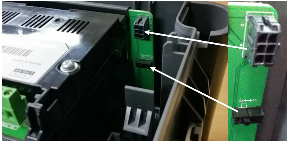
Figure 37. Battery On/Off Switch and Battery Connector
