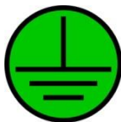
Figure 3. Protective Earth (Ground) Point
