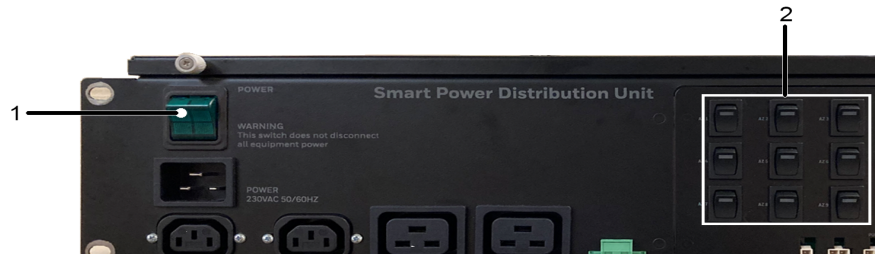
1) Main Power ON/OFF Switch, 2) Analyzer Power Switches
