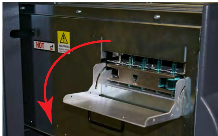
Figure 5-5. Pyrolyzer Filter Door
