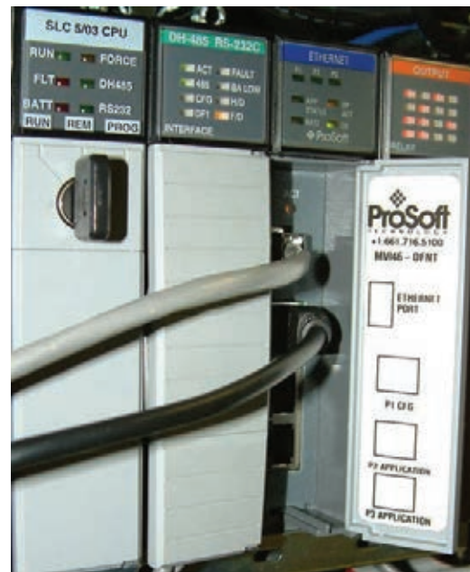
Figure F-6 -- Connector Locations
